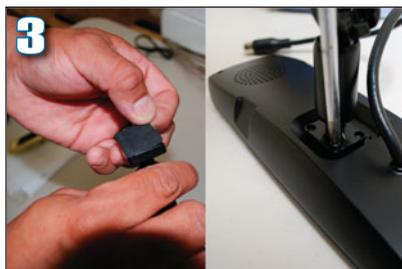
**3** Prep the navigation mirror. Attach the adhesive pad to the mirror stem, lining up the holes. Secure the stem to the back of the mirror with the supplied washers and screws, starting with the holes nearest the top of the mirror housing.
