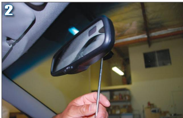
**2** Remove the old mirror and unplug if necessary. The mirror is usually attached by a single screw. If a wire harness was attached, stuff it behind the headliner. It will not be used with the new mirror.
