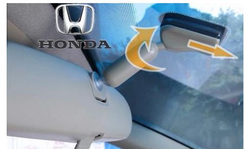
**NOTE:** If the Rydeen Mirror does not fit the mount on your windshield, it is possible that one of our adapter plates may. It may also be possible that the mirror button will have to be replaced with one that is compatible with the Rydeen Mirror (example: Fords built prior to 1996). If you need information concerning one of Rydeen adapter plates or a mirror mounting kit, please call 1-877-777-8811 and speak with Rydeen sales or technical support agent.
