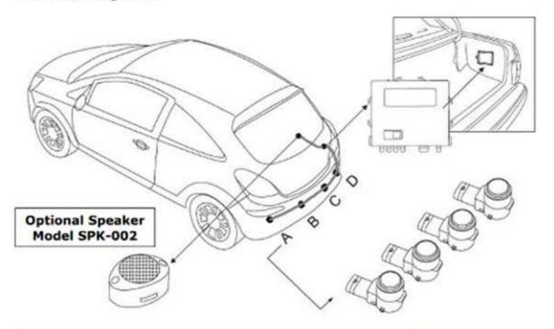
Place the speaker and control box inside a vehicle. Avoid from water damages. The speaker or buzzer sound will indicate the distance between the sensors and the object. Shorter pitch tone sound indicates getting closer to objects.
