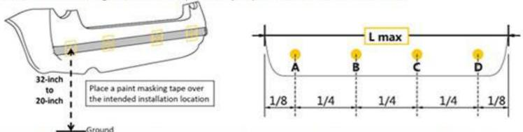
3) Generally, it is the best to mount the sensors as high as possible in the bumper. Use paint masking tape and mark the location as above diagram for the proper spacing of the sensors.
