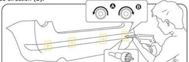
BB-420P sensors <u>MUST be installed inside the bumper plastic skin</u> and only the sensor head to exposed to outside. <u>Bumper removal is required for this installation.</u>
